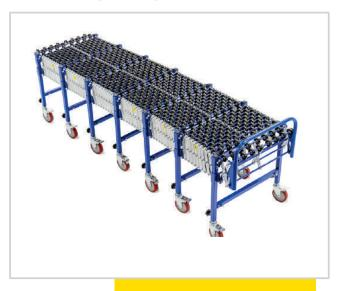
Flexible skate wheel Conveyor convey lightweight loads that have firm flat bottoms such as cartons, totes, cases, etc. Skate wheel conveyor "rolls" more easily than roller conveyor allowing for lighter packages and less slope. The individual wheels in the curve sections allow packages to track more so than roller conveyor.
